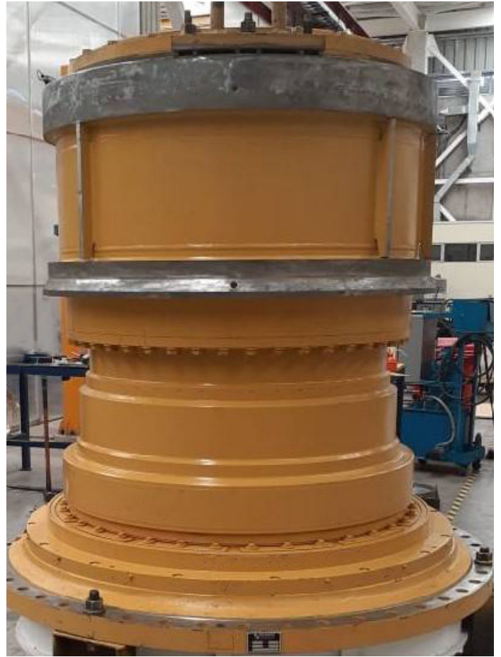
Birrana™ remanufactured 830E wheel motor
