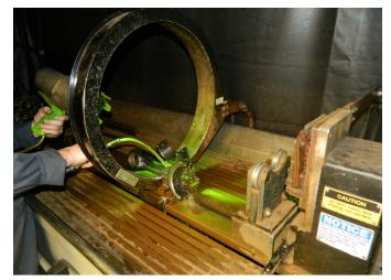
Connecting Rod Magnetic Particle Inspection (NDT)
