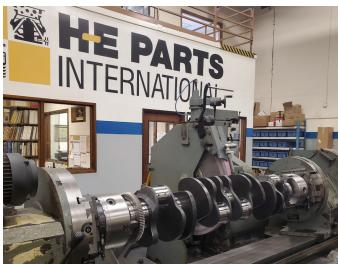
Crankshaft Set Up for Grinding
