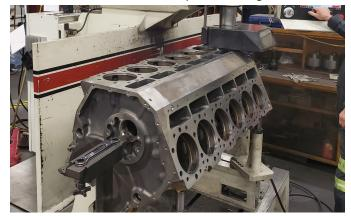
Machining Cylinder Block Surface
