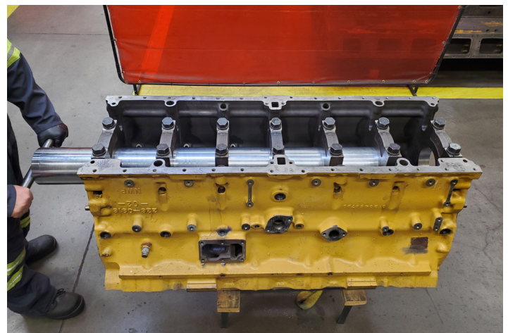
Confirming Proper Main Bearing Bore Alignments
