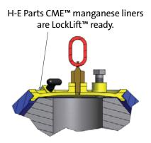
Locks in above the pouring hole. Backing can't interfere with the lifting process.
