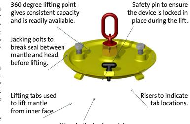
Wear indicator to assist checking lifting safety of worn liners.
