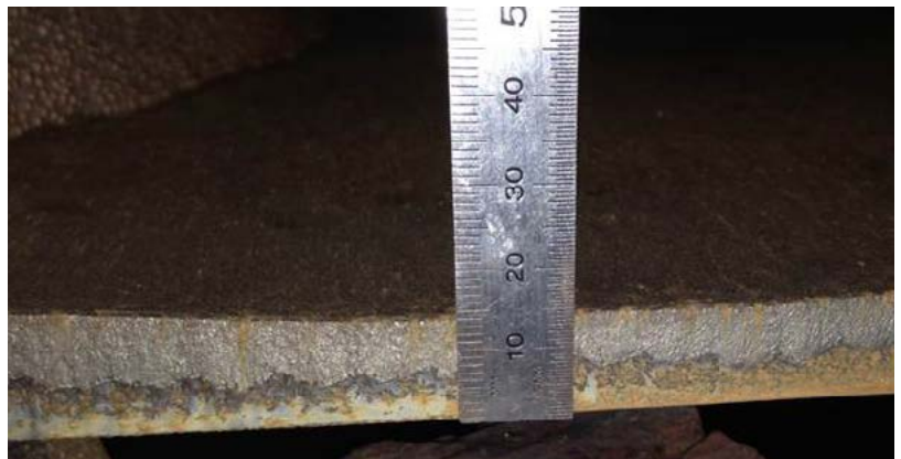
Competing plate after 2 weeks - 4mm of wear
