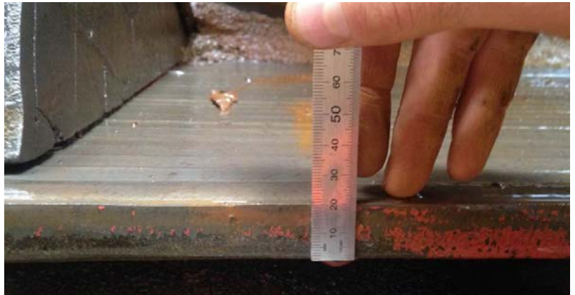
CME™ overlay liners after 2 weeks - no wear
