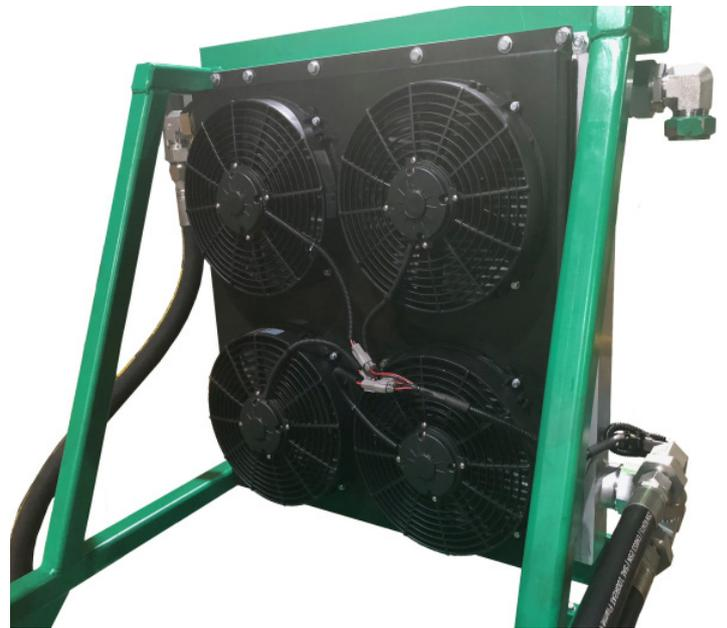
H-E Parts replaced the radiator core with a more efficient core that allows for a larger cooling capacity with better airflow. In combination with the radiator re-build, H-E Parts worked closely with Multi-Wing to redesign a suitable replacement fan that provides higher airflow. The radiator and fan combination work better to achieve a more efficient cooling solution, better suited to Australia's ambient temperatures of 50 °C / 122 ° F.
